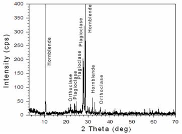
Fig. 1. XRD profile of the natural raw material sample and mineral phases identified
