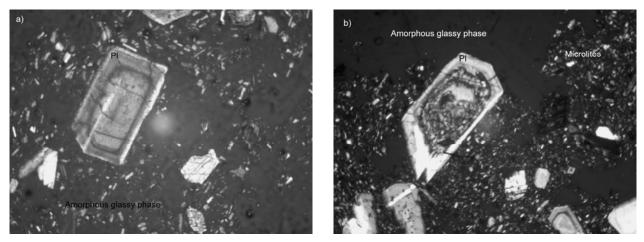
Fig. 3. Microscopic observations under polarized light (x10, XPL). a) A phenocryst of zoned plagioclase and b) a phenocryst of plagioclase (Pl) with a sieve texture
