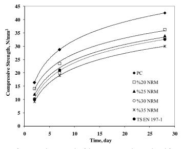
Fig. 4. Development of compressive strength of the mortar samples produced from blended cements containing up to 35% w/w natural raw material over a curing period of 28 days
