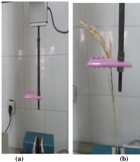
Fig.3. (a) A simple tool was used to measuring tensile force; (b) Display the snapping of the grains paddy from the cluster by shoulder.
