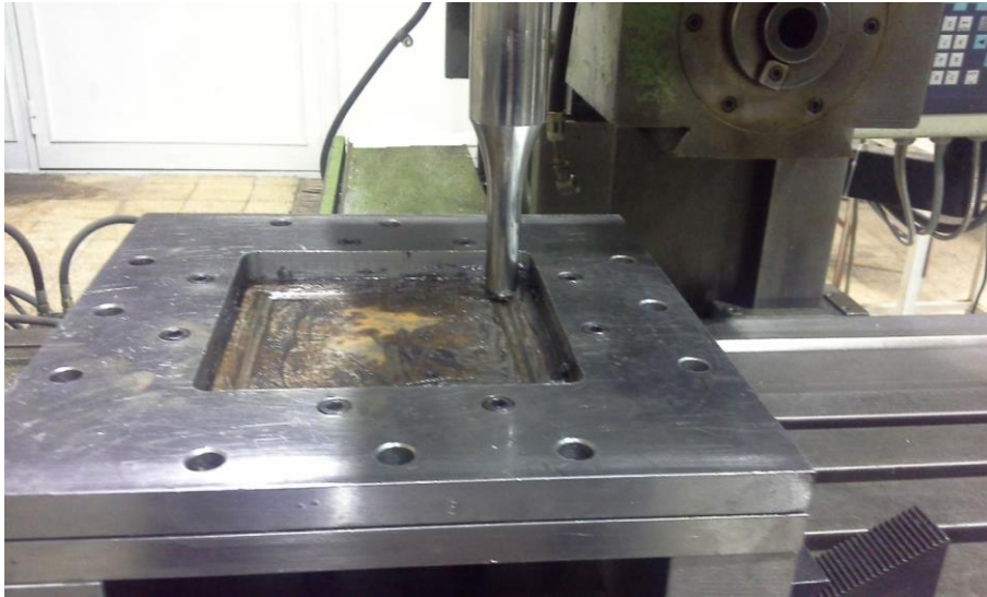
Fig. 6. Formation of a pyramidal specimen during the process.
