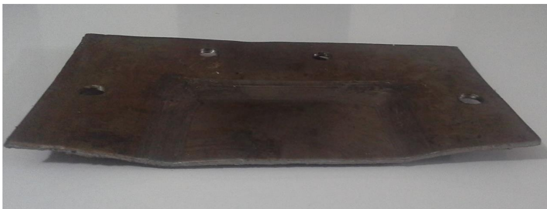
Fig. 13. The pyramidal specimen to evaluate the thickness distribution.
