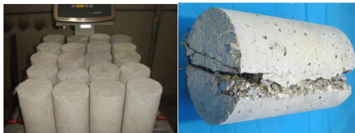
Fig. 6. Cylinder specimens for splitting test and Failure mode of specimens
