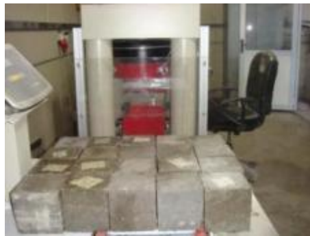
Fig. 2. Concrete specimens for compressive strength test
