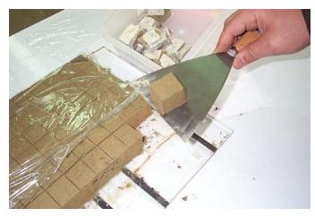
Fig. 2. Slicing the soil samples after termination of the 2-D diffusion tests
