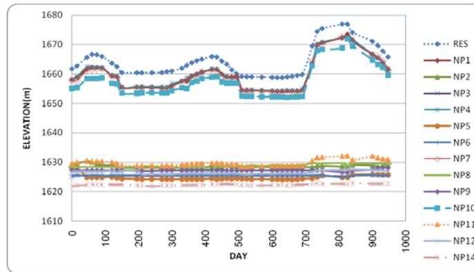
Fig. 6. Reservoir and piezometric level observations used for model calibration
