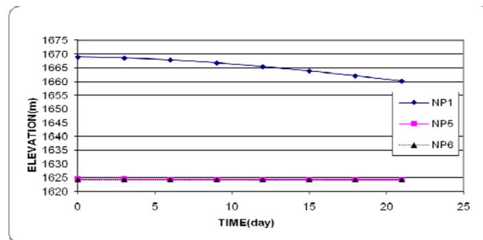
Fig. 10. Total head variation during rapid drawdown at the dam upstream and downstream locations
