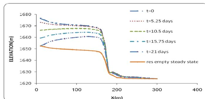
Fig. 11. Phreatic line dynamics during rapid drawdown and at steady state at section A-A
