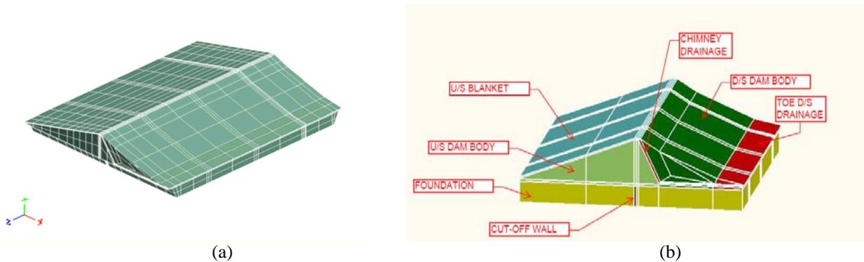
Fig. 5. (a) Doroodzan dam 3-D finite element model, (b) dam body components
