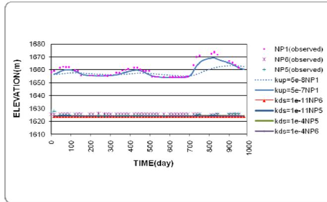
Fig. 7. Observed and simulated elevations at piezometers NP1, NP5, NP6 for two upstream ( $K_{up}$ ) and two downstream ( $K_{ds}$ ) hydraulic conductivities (in  $m/s$ )
