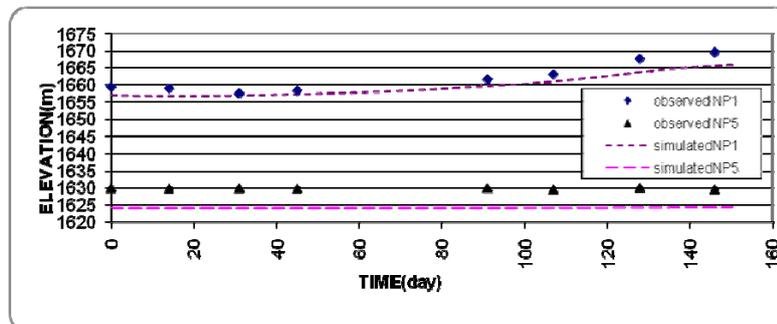
Fig. 9. Verification results based on observed and simulated elevations at NP1 and NP5
