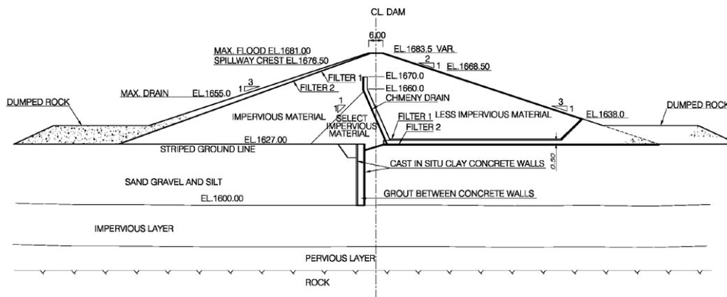
Fig. 2. Cross Section A-A of Doroodzan Dam (the cross section is shown on Fig. 4)
