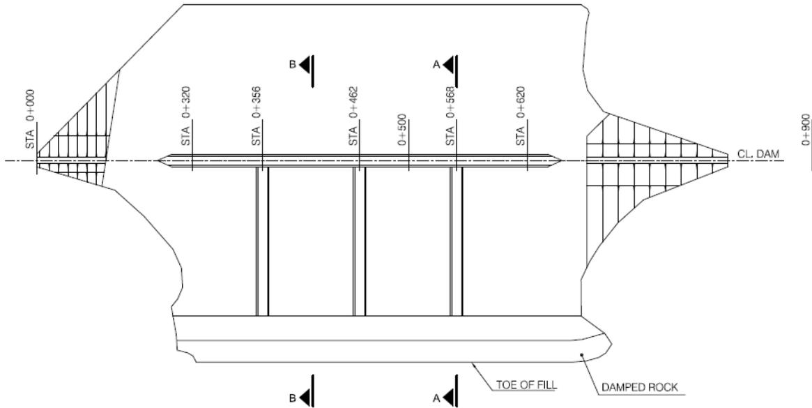
Fig. 4. Doroodzan dam horizontal and vertical drainage locations
