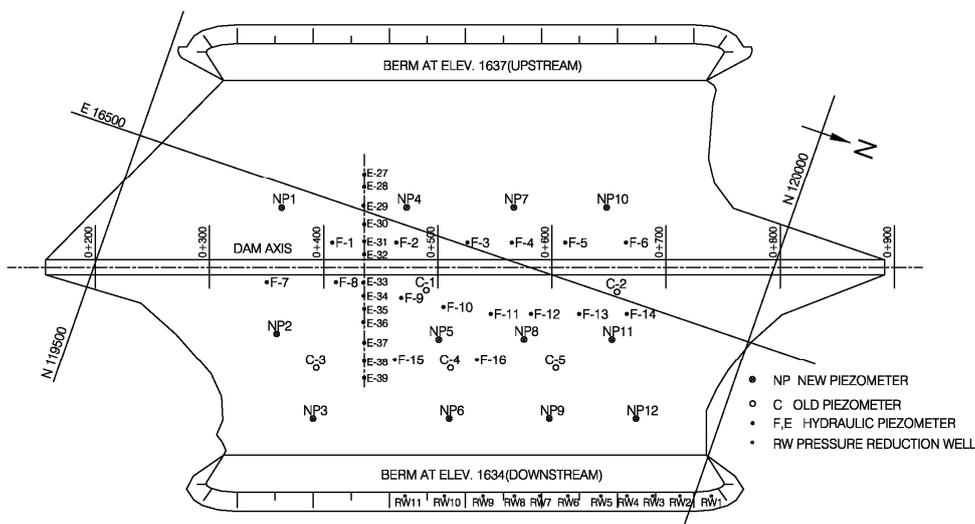
Fig. 3. A plan view of piezometers location in Doroodzan dam
