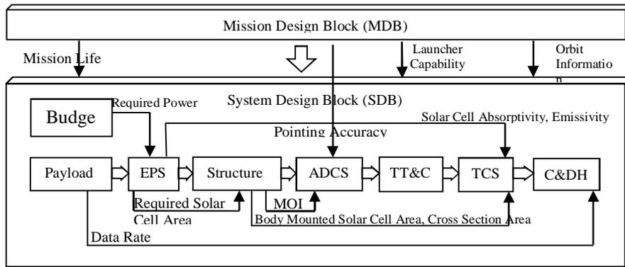
Fig. 2. Elements of a typical satellite system design
