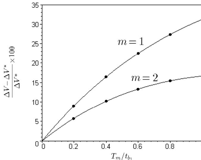
Fig. 6. Percent increase of  $\Delta V$  vs time margin for  $t_{b_1} / t_f = 1 / 4$
