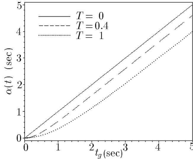
Fig. 3. The value of  $\alpha(t)$  for single-lag autopilots
