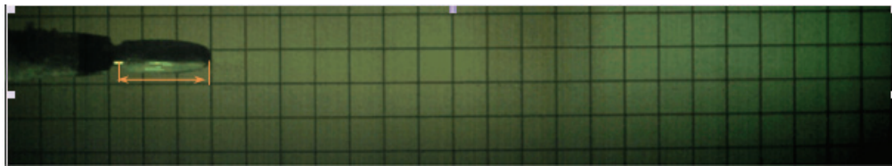
Fig. 10. Measurement of bubble length in partial cavitation
