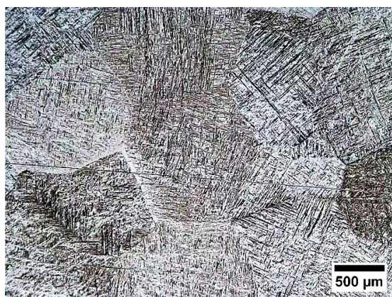
Fig. 4. Microstructure of Ti-6Al-4V alloy after \beta annealing treatment (point A in Fig. 2).
