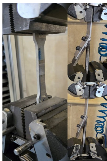
Fig. 11. Tensile testing setup showing the specimen mounted inside the wedge grips of the universal testing machine during axial loading.
