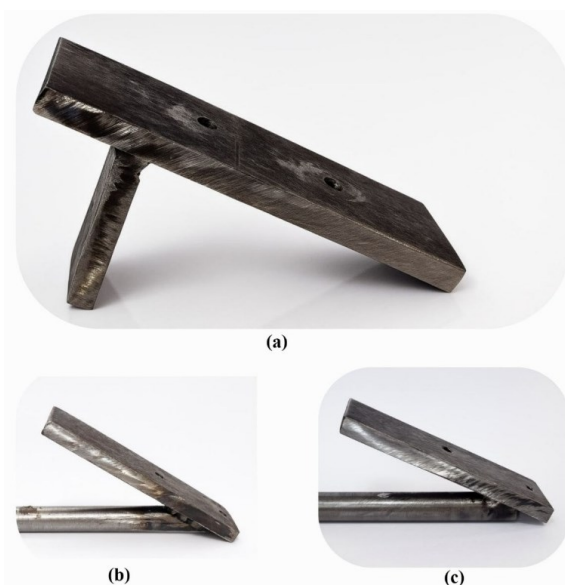
Fig. 10. Tensile testing fixtures fabricated for the angled FSW configurations: (a) 90°, (b) 150°, and (c) 165°.
