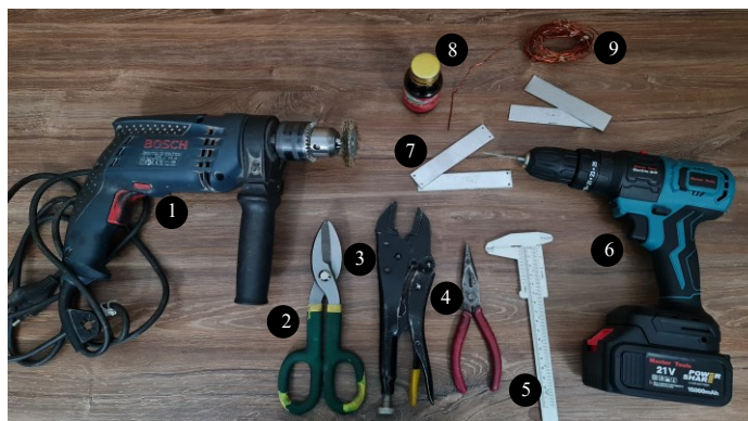
Fig. 2. Tools and materials used for surface preparation prior to ARB: (1) handheld mini-grinder with a steel wire brush (wire diameter: 5 mm, 750 rpm); (2) scissors for cutting rolled sheets; (3) pliers for holding sheets during drilling and brushing; (4) needle-nose pliers for tightening copper wires; (5) caliper for thickness measurement; (6) handheld drill for hole drilling at the sheet corners; (7) primary aluminum sheets (initial strips); (8) acetone for degreasing (30 s immersion); (9) copper wires (0.6 mm in diameter) for fastening the stacked sheets.
