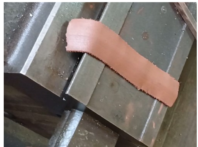
Fig. 17. Clay extrusion output from the optimized die.
