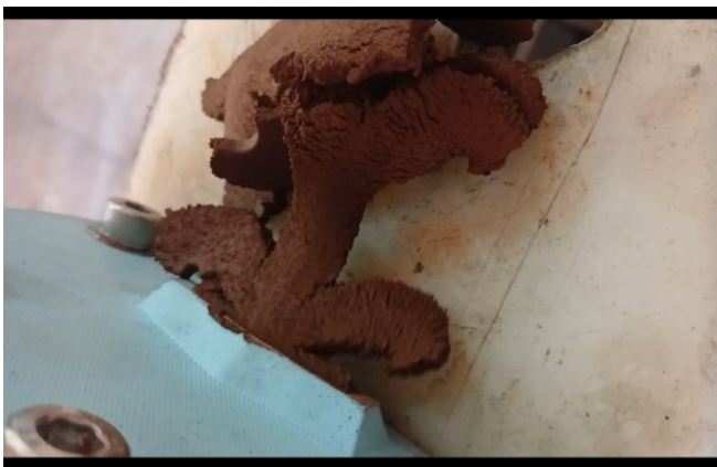
Fig. 15. Clay extrusion output from the non-optimized die.
