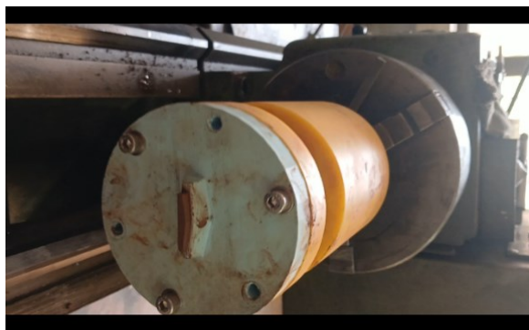
Fig. 7. The mounting mechanism of the physical simulation apparatus within the lathe system.
