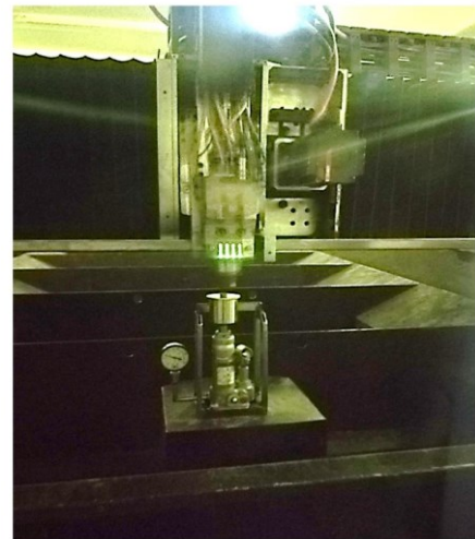
Fig. 4. Placing the auxiliary force mechanism and blank on the laser machine.
