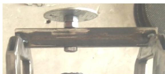
Fig. 2. The location of the workpiece clamp on the fixture.
