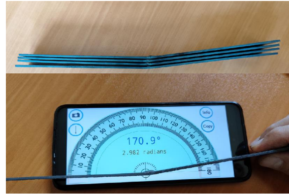
Fig. 1. Bending of specimens due to residual stress induced by welding.
