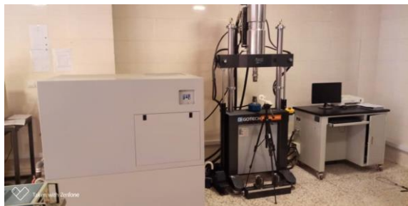
Fig. 2. Fatigue testing machine used for conducting the fatigue crack growth rate tests.
