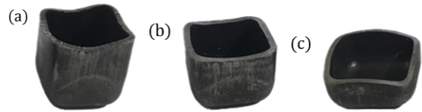
Fig. 6. Cups formed by experimental tests from blank with diameters of (a) 75 mm, (b) 65 mm, and (c) 55 mm.
