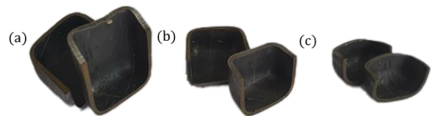
Fig. 7. Samples of cut pieces by wire cut blank with diameters of (a) 75 mm, (b) 65 mm, and (c) 55 mm.
