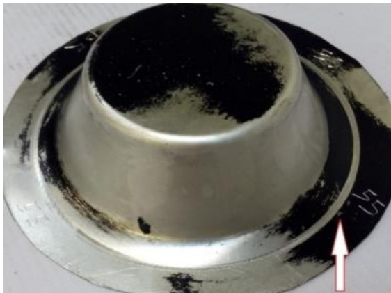
Fig. 6. Visibility of sheet displacement inside the die during forming.
