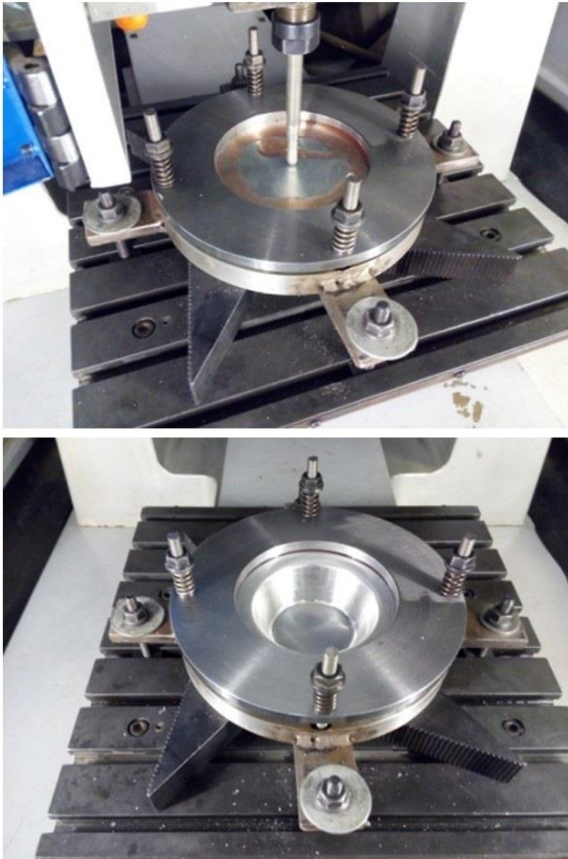
Fig. 4. Installation of the specialized SIF tooling set on the milling machine.
