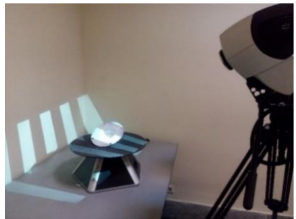
Fig. 7. Scanning of the formed parts using a 3D scanner.
