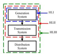
Fig. 2. Electric power system hierarchical level diagram [7].
