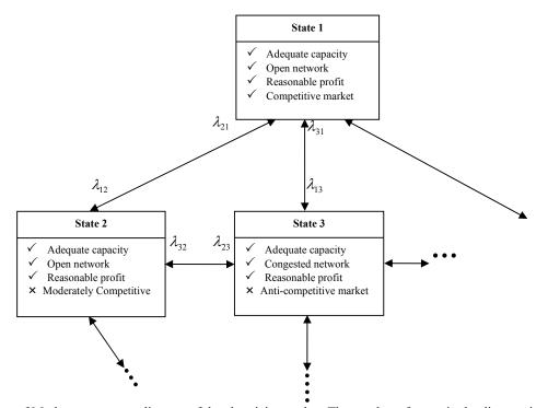
Fig. 6. Part of Markov state space diagram of the electricity market. The number of states in the diagram increases as the number of market performance indices increases and the number of states in which each index can reside increases. If n + m indices are considered, the number of states in the diagram are  $2^n \times 3^m$  where n is the number of 2-state indices and m is the number of 3-state ones
