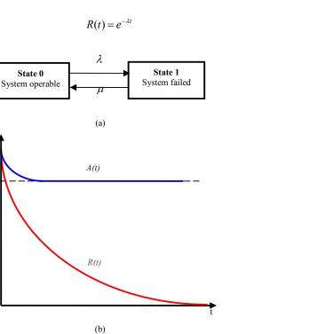
Fig. 5. Repairable system: a) State space diagram. b) Variation of reliability and availability [3]
