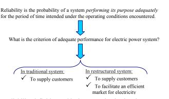
Fig.1. Reliability definition and its interpretation in electric power system
