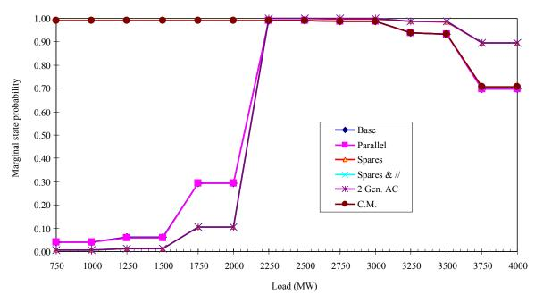
Fig. 5b. System marginal state probabilities for the HVDC transmission system
