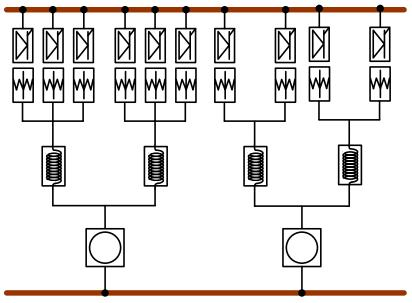
Fig. 2a. HVDC reliability diagram
