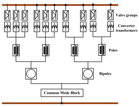
Fig. 2b. HVDC reliability diagram (including common mode failures)
