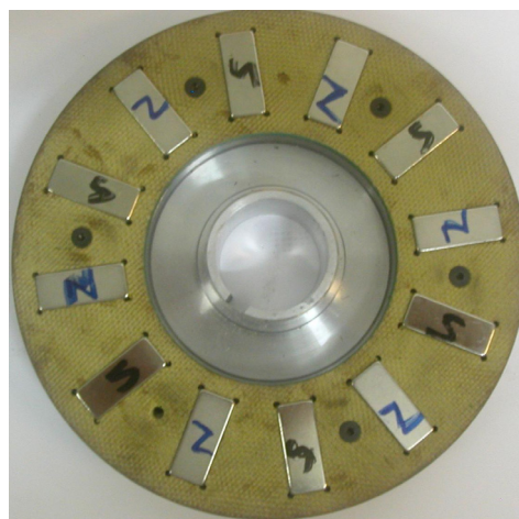
Fig.10. A rotor disk with magnets and non-ferromagnetic holder
