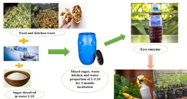
Fig. 2. Eco-enzyme production process.
