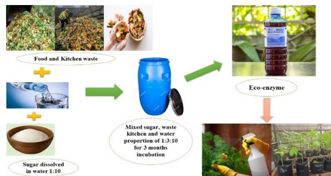
Fig. 2. Eco-enzyme production process.
