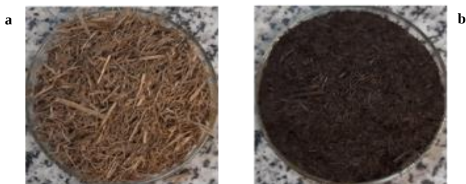
Fig. 2. Samples. (a) Sugarcane bagasse and (b) biochar of sugarcane bagasse.
