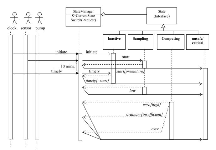
Fig. 9. The event tracing sequence diagram of violations in the CIIP system
