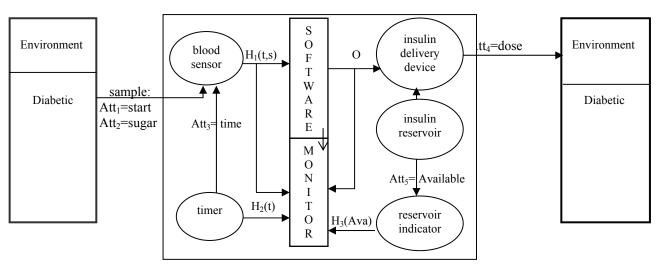
Fig. 7. The CIIP system model
