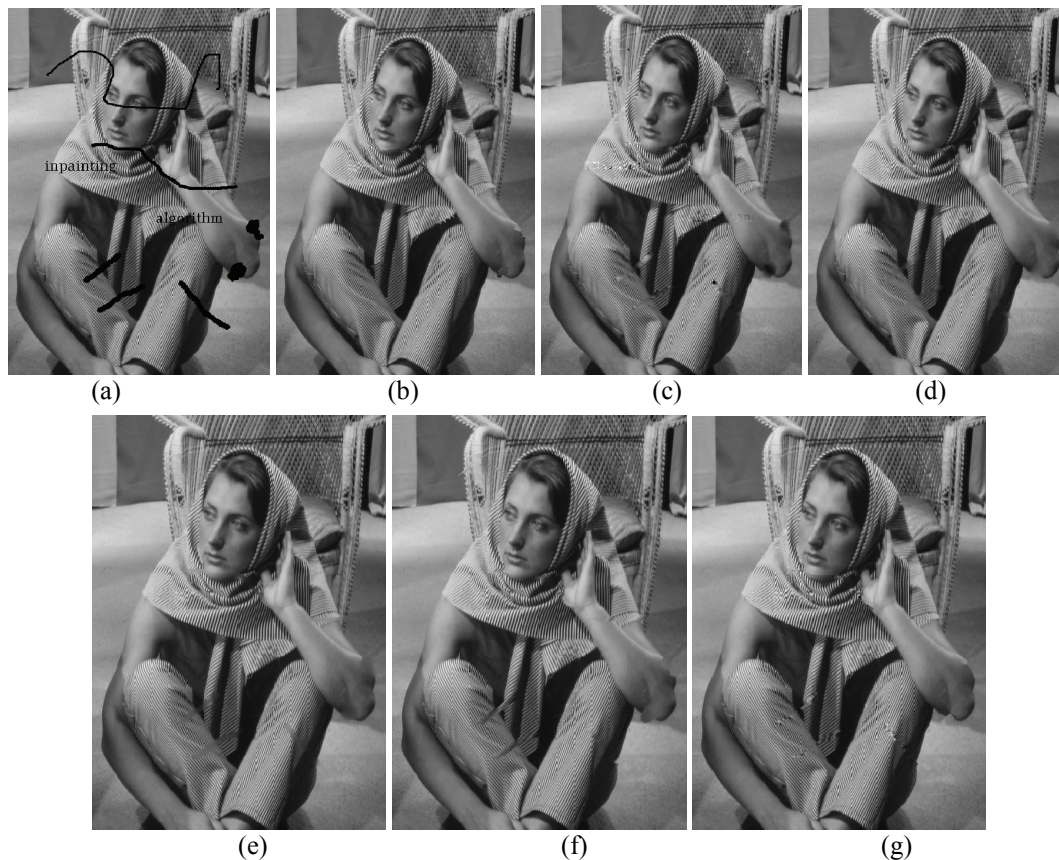
Fig. 15. a) damaged image b) inpainted with Efron model c) Bertalmio's algorithm result d) restored by Oliveira method e) result of TV algorithm. f) result of Bornemann's approach. g) proposed algorithm result with \sigma_d=0.5 and \sigma_r=25.5 and 2 iterations for texture regions and 80 iterations for structure regions
