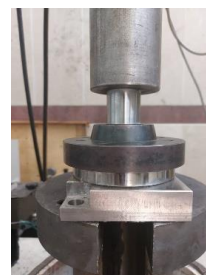
Fig. 6. Nakazima FLD dies under press.
