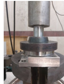
Fig. 6. Nakazima FLD dies under press.
