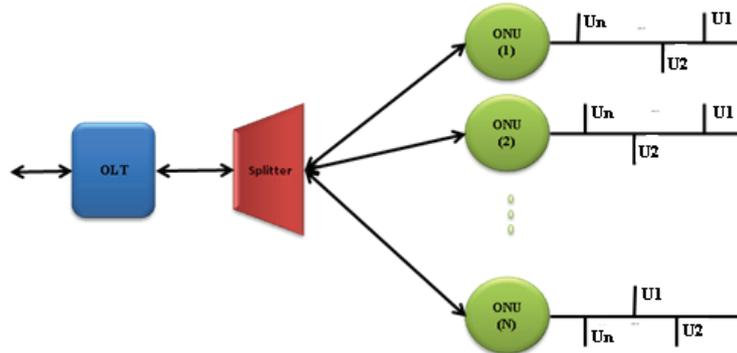
Fig. 1. EPON's architecture
