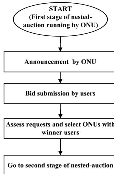
Fig. 3. Overall design of nested-auction's first stage in the proposed Parnian method
