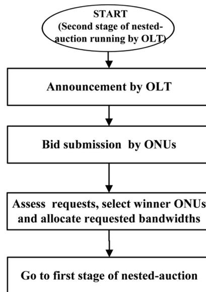
Fig. 6. Overall design of the second stage of nested-auction in the proposed Parnian method
