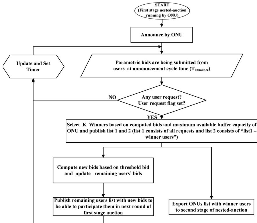
Fig. 5. Overall execution process in the first stage of nested-auction
