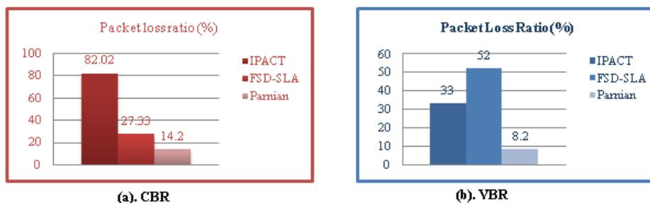
Fig. 10. Comparison of packet loss ratio in FSD-SLA, "limited service" IPACT, and Parnian
