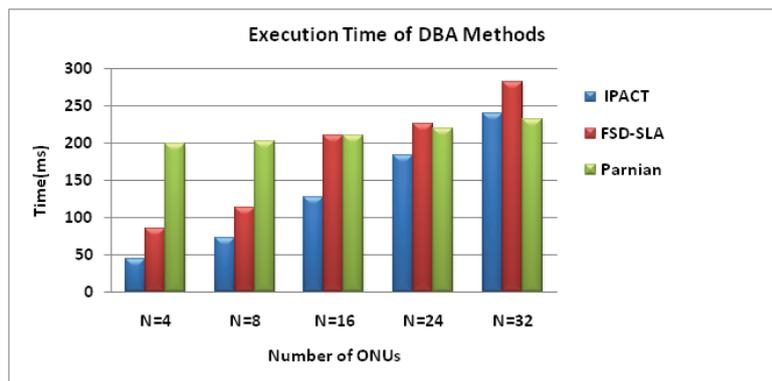
Fig. 13. Comparison of Execution Time in FSD-SLA, "limited service" IPACT and Parnian
