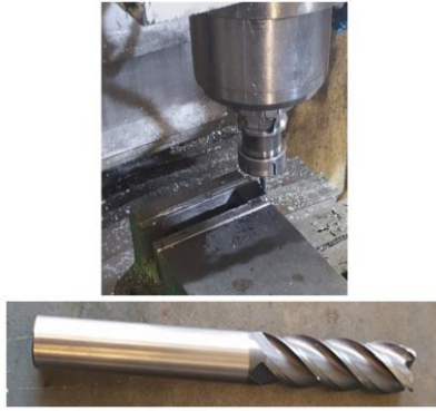
Fig. 2. Milling procedure for preparing the upper step surface of the workpiece.
