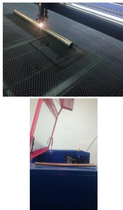
Fig. 1. The experimental setup of the laser tube forming process and the resulting laser formed tubes.
