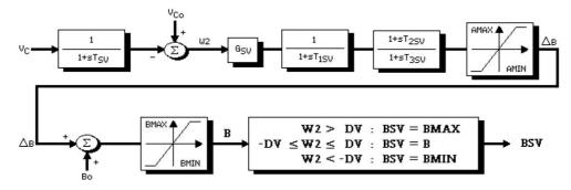
Fig. 6. SVC controller diagram in the M.S.C power system
