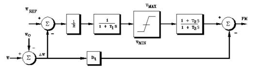
Fig. 4. Governor system for steam generator units in the M.S.C and E.R.E.C network
