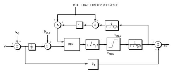
Fig. 5. Governor system for gas generator units in the M.S.C and E.R.E.C network
