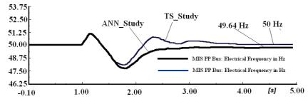
Fig. 11. Frequency response of M.S.C system in two different algorithms in different case 4
