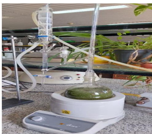
Fig. 1. Extracting essential oils from the Froriepiea subpinnata plant using a Clevenger apparatus.
