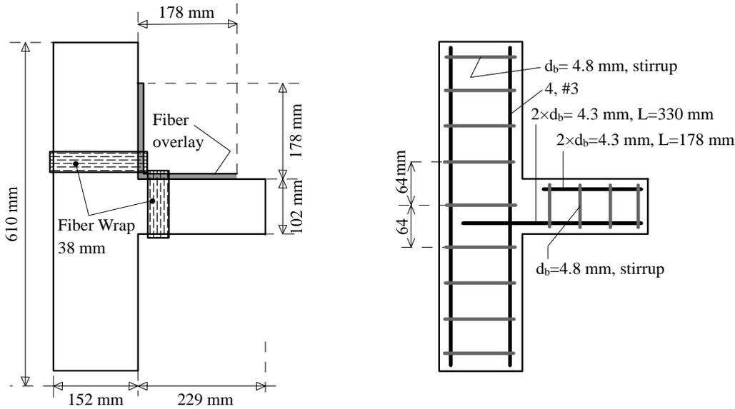
Fig. 4. Reinforcement specification of the RC joint and FRP strengthening plan [3]
