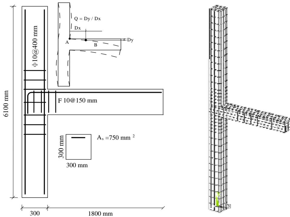
Fig. 1. Specification of the selected RC joint and its FE mesh
