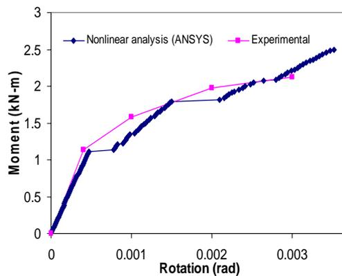
Fig. 5. Moment-rotation curve for the joint in Fig. 4 extracted from experiment [3] and calculated from FE analysis
