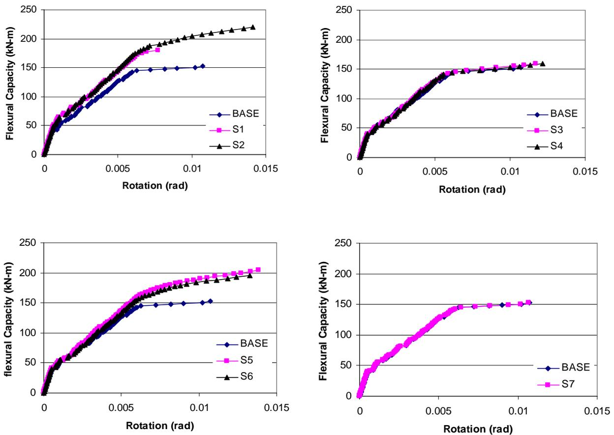
Fig. 7. Moment-rotation curves for the base specimen and the strengthened specimens (extracted from non-linear analyses)
