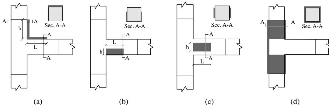
Fig. 6. Strengthening designs with FRP overlays
