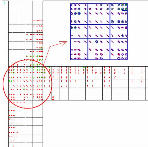
Fig. 8. Pattern of cracks in the joint under ultimate load and the consecutive shear failure of the joint
