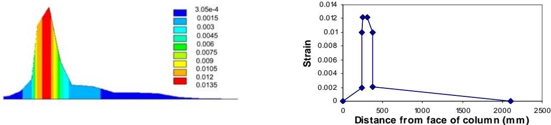
Fig. 3. Strain variations in longitudinal tensile reinforcement of the beam resulted from FE and theoretical analyses
