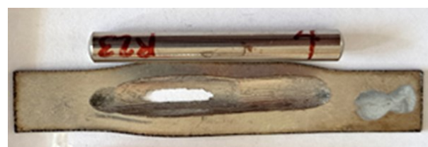
Fig. 6. Influence of path length of 500 m on the metal friction.
