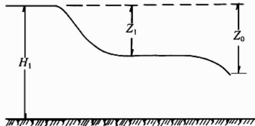
Fig. 3. Flow state of outburst flood.  $H_1$  is the water depth at the dam before failure;  $Z_1$  and  $Z_0$  are values of water-level fall after dam failure
