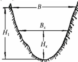
Fig. 1. Sketch of gully cross-section.  $B_x$  is the flood width after dam failure;  $B$  is the failure channel width;  $H_x$  is the flood height after dam failure;  $H_1$  is the water depth at the dam before the failure
