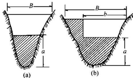
Fig. 2. Partial burst of a debris dam.  $B$  is the failure channel width;  $b$  is the width of the partial outlet;  $a$  is the height of the remaining dam
