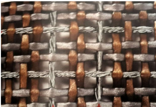
Fig. 9. Fabric reinforced with steel wires [22].
