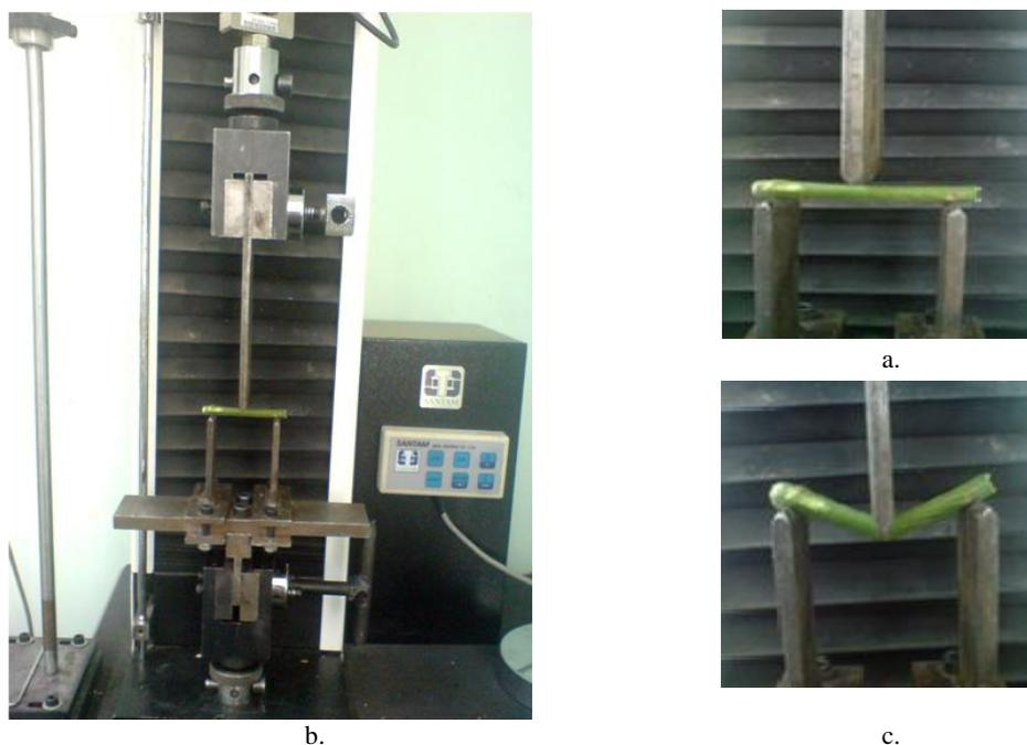
**Fig.2.** a. The sample before fracture, b. The Instron Universal Testing Machine (STM-5) with attached bending device, C. The sample after fracture
