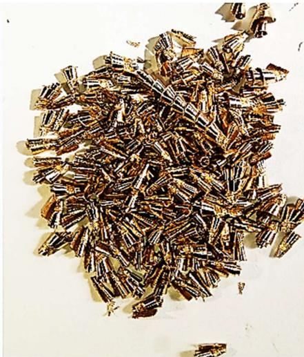
Fig. 1. Brass chips employed in this investigation to make brass wire.
