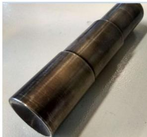
Fig. 2. The FSBE tool used in this investigation.
