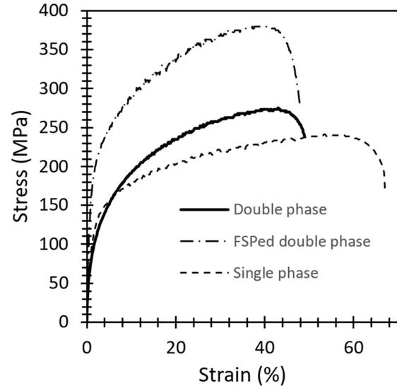
**Fig. 6.** Stress-strain plots for different samples before heat treatment (single phase), after heat treatment (double phase), and after FSP.
