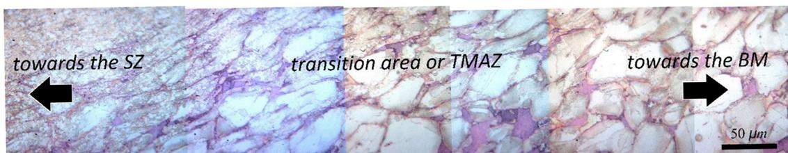
Fig. 2. Combined OM image of the transition area in advancing side of the friction stir processed sample form BM to SZ.
