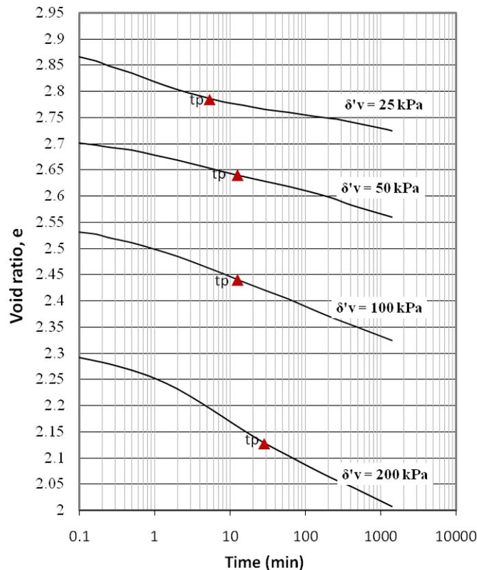
Fig. 5. Void ratio versus logarithm of time curves for Urmia peat with 33% of organic content
