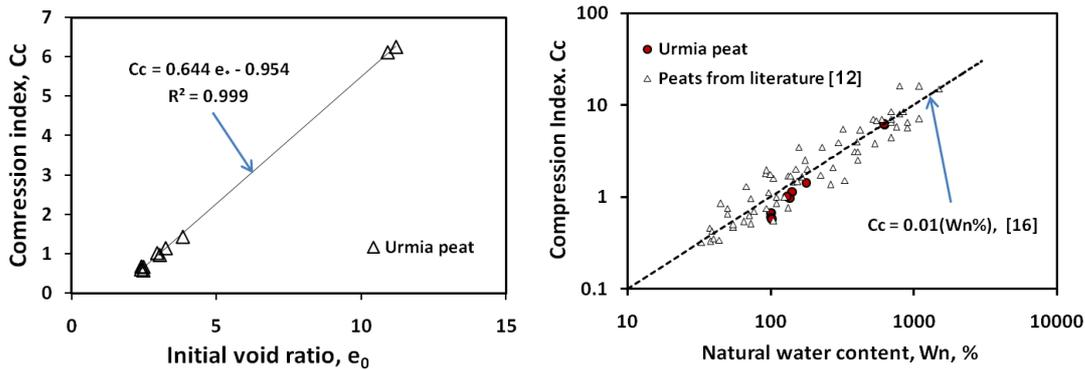
Fig. 10. Relationship between, (left) compression index and initial void ratio, (right) compression index and natural water content
