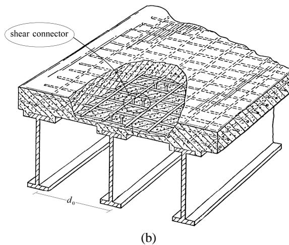
Fig. 1. Schematic view of (a). variables of composite floor system, (b). a simple composite floor system
