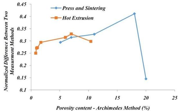
Fig. 8. Normalized differences between porosity measured by image analysis method relative to Archimedes method.
