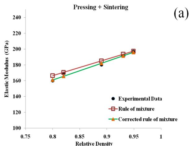
Fig. 11. Comparison between experimental and calculated elastic modulus according to the equation 2 and 3 for (a) Group I and, (b) Group II specimens.
