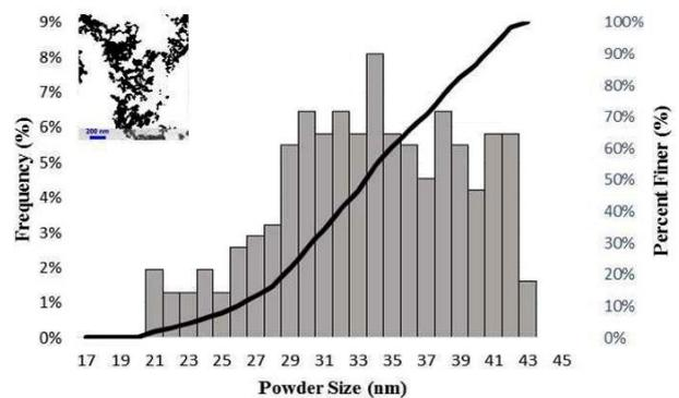
**Fig. 1.** Size distribution of the yttrium oxide particles.
