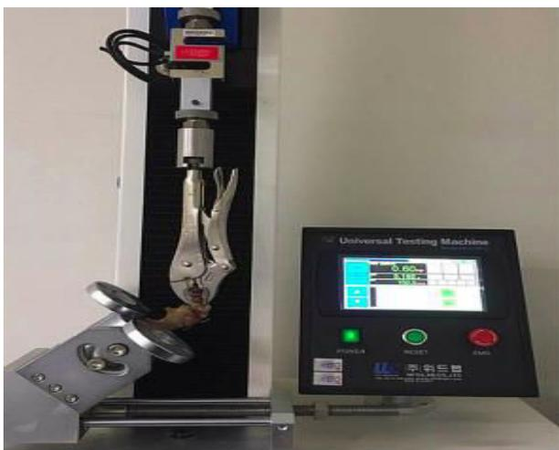
**Fig. 4:** Fixation of the specimen in a frame that the long axis of the ulna positions at an angle of 135° from the vertically aligned triceps tendon. The parameters are based on the mean and standard deviation
