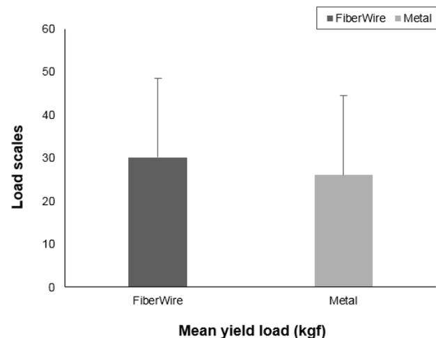
**Fig. 6:** No significant difference was observed, but the mean yield load (MYL) is higher when using No. 2 FiberWire (31.345 kgf) is used as tension bands than when 0.76 mm metal wire (27.070 kgf) is used
