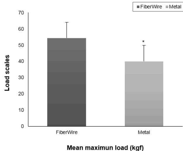
**Fig. 5:** The mean maximum load (MML) is significantly higher when using No. 2 FiberWire (54.330 kgf) as tension bands than when using 0.76 mm metal wire (43.365 kgf). \*  $P<0.05$
