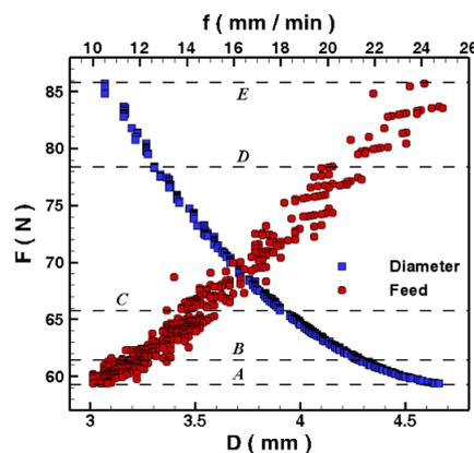
Fig. 6. Optimal variations of force with respect to design variables ( $f$  and  $D$ ).
