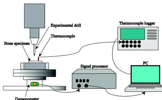
Fig. 1. Bone drilling process and temperature measurement in the absence of cooling system.
