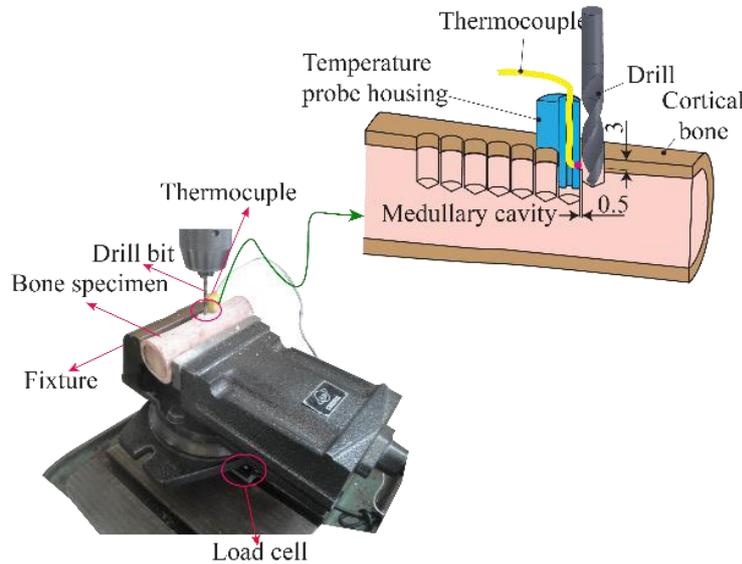
Fig. 2. Experimental Setup and Thermocouple positioning in bone drilling process.
