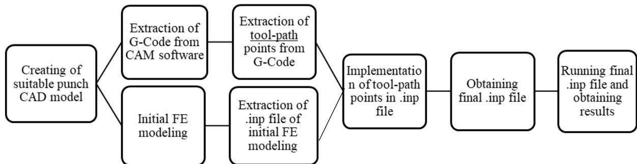
Fig. 2. General workflow of FE modeling and used software.
