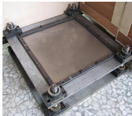
Fig. 7. Configuration of experiment of TPIF for saddle-like part.
