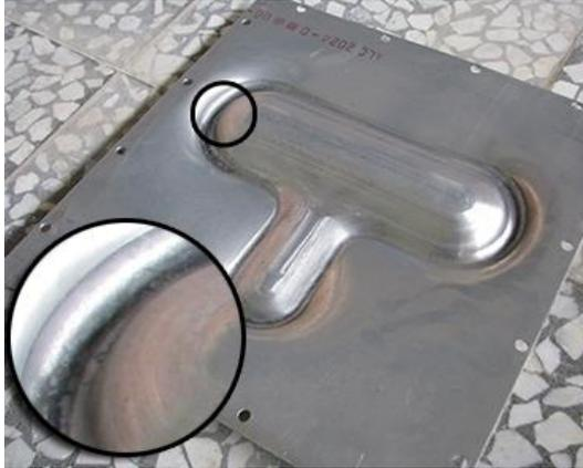
Fig. 11. Tearing seen in sheet, when tool has come down by 34mm.
