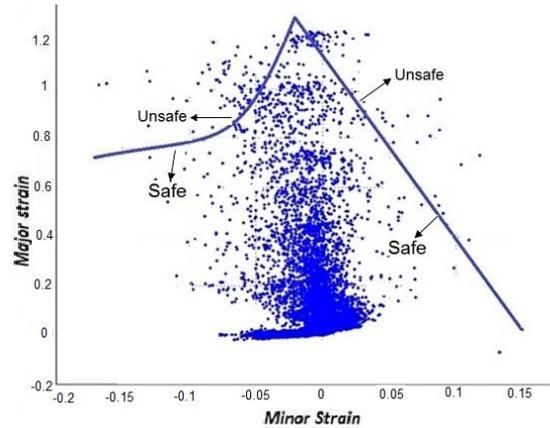
Fig. 12. Comparing the values of [major strain, minor strain] in deformed sheet with forming limit diagram when tool has reached the depth of 34 mm.
