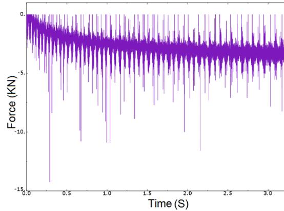
Fig. 9. History of the force exerted on the tool in depth direction obtained from simulation.
