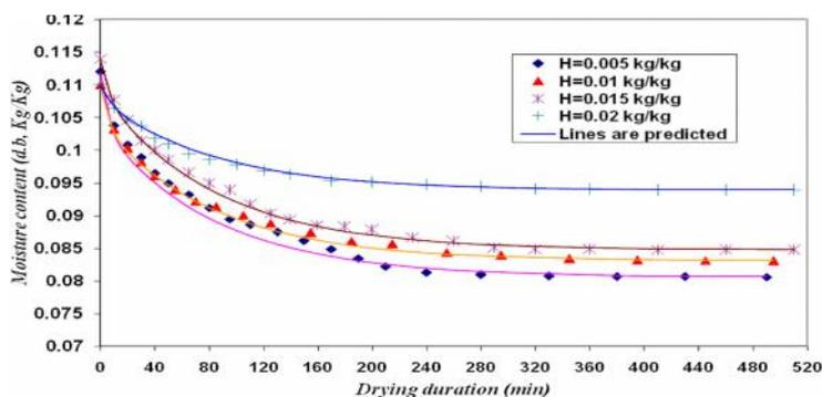
Fig. 4. The drying trend of canola for different drying air humidity levels at constant air temperature of 45°C
