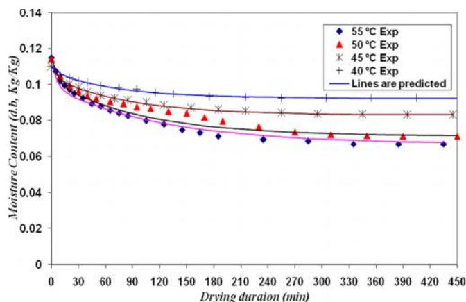
Fig. 3. The drying trend for different drying air temperatures at constant absolute humidity of 0.01Kg/Kg
