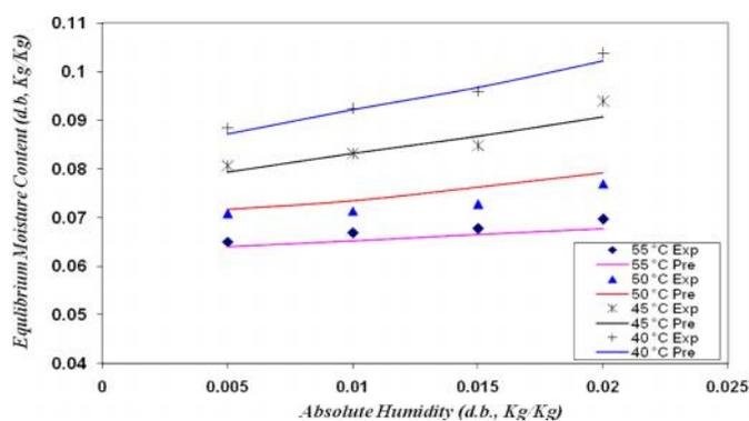
Fig. 5. The isotherm equilibrium moisture content of experimental data and those predicted by the modified Smith model
