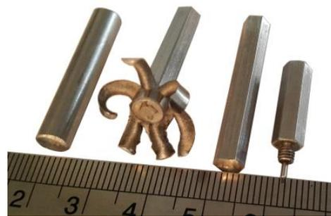
Fig. 18. Round bar, hexagonal bar made by AISI M42, hexagonal bar with micro machining
