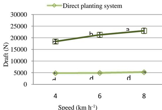
**Fig. 5.** Effect of cropping system and speed on the average draft force
