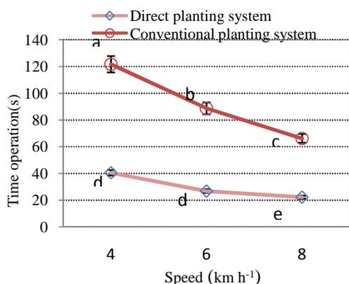
**Fig. 3.** Effect of cropping systems and speed on the average values of operations time
