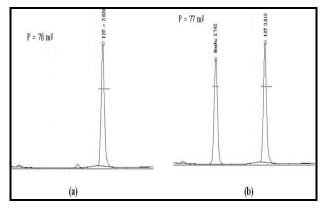
**Fig. 1:** Representative chromatograms of marbofloxacin and sarafloxacin. (a) Blank plasma spiked with 16  $\mu$ g/ml of sarafloxacin, and (b) blank plasma spiked with 16  $\mu$ g/ml of sarafloxacin and 16  $\mu$ g/ml of marbofloxacin
